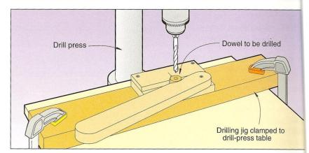
I built a game scorekeeper that uses short lengths of dowel that slide on a rod, similar to an abacus. I cut the dowel sections first, then figured out a way to drill the holes in the thin "slices". My solution was to build the jig, shown *above*.
